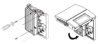
**NOTE:** If necessary, before re-installing the front component, configure the thermostat (see section 3).
